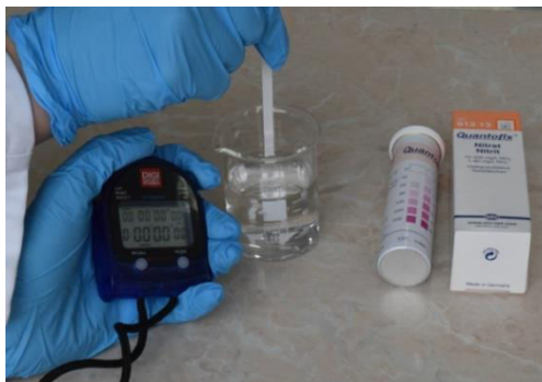
Fig. 1 Experimental setup to determine \text{NO}_3^- and \text{NO}_2^- in drinking water.
