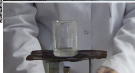
Fig. 4 If the solution is cooled down straight away crystals will not form, but a paste form will be observed.
