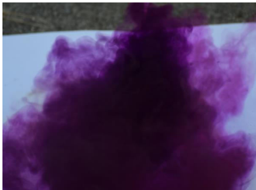
Fig. 3 The I_2 sublimates due to the heat evolved on the reaction site.
