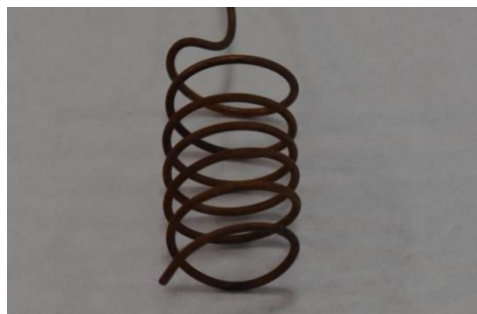
Fig. 1 Oxidized copper wire after heating in oxidizing flame before immersing in ethanol.
