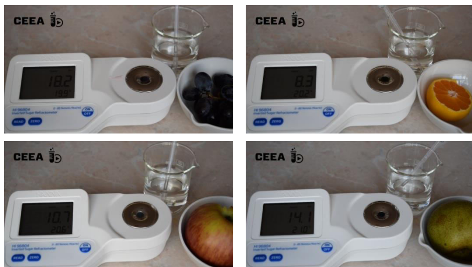
Fig. 1-4 Some common fruits and their sugar content measured with a refractometer. (from left to right grapes, clementine (up), apple and pear (down))
