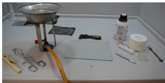
Fig. 1 HF is lighter than air and diffuses in air easily, so the experiment must be conducted in a fume hood.
