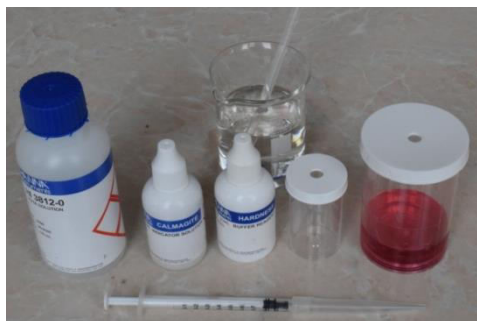
Fig. 1 At the beginning of the experiment the indicator Calmagite is red due to its complexation with \text{Ca}^{2+} and \text{Mg}^{2+} ions.
