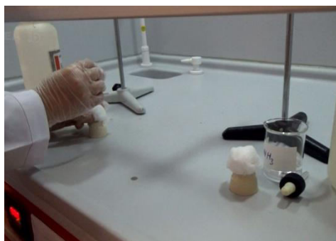
Fig. 1 Due to HCl and \text{NH}_3 being toxic and spreading very quickly this experiment must be conducted in a fume hood.
