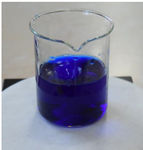
Fig. 1 The Schweizer's Reagent as the only solution capable to dissolve cellulose.
