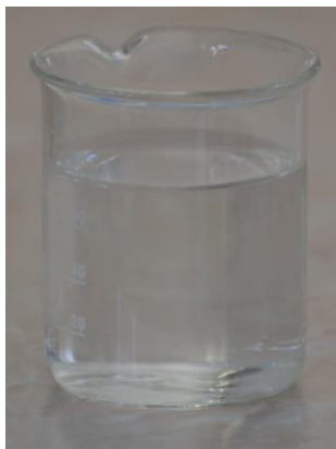
Fig. 1 Clear colorless solution of HgCl 2 having the volume ~70 mL, the starting reagent of the Nessler solution.
