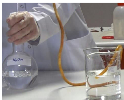
Fig. 4 When formic acid is added to the solution consisting of \text{NaOH} , it is observed that no gas release happens.
