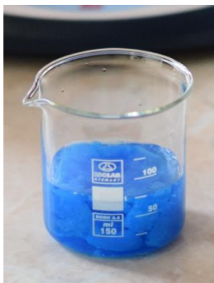
Fig. 2 Abundant precipitate of \text{Cu}(\text{OH})_2 obtained by the addition of 1M NaOH solution to the copper salt.
