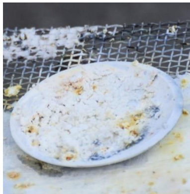
Fig. 4 The white end product, ZnS known also as white pigment is yellow when still hot.
