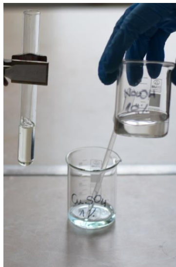
Fig. 2 Add to the protein solution in the test tube the same volume of 10% NaOH.
