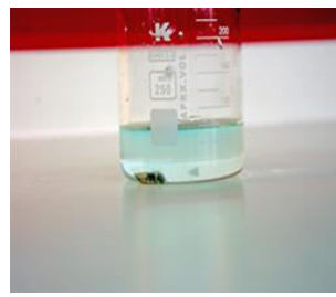
Fig. 3 The colourless solution of \text{AgNO}_3 turns into a characteristic blue as the concentration of copper ions builds
