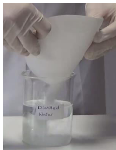
Fig. 1 When preparing solution A, we add 20g of iodine free salt into distilled water.
