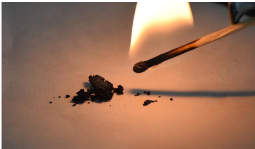
Fig. 3 A small amount of silver acetylide (three times the size of a match head) is capable to produce a loud bang when ignited from a safe distance.
