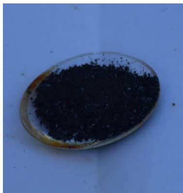
Fig. 1 Mixture of Mg and I 2 prepared carefully by mixing both reagents on a sheet of paper.
