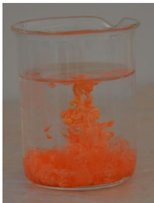
Fig. 2 Insoluble orange HgI 2 start to precipitate when adding to the HgCl 2 a saturated solution of KI.
