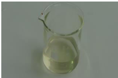
Fig. 2 The filtrate after filtration. Some sand particles penetrated the pores of the filter paper for this reason, the filtrate is not completely clear.
