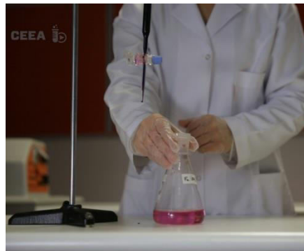
Fig. 4. The shaking is ended when the solution turns into a stable pink color.
