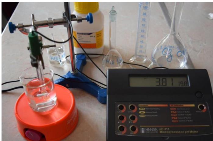
Fig. 1 Experimental setup for measuring the buffer properties of amino acid solutions (0.1M) when strong acid is added. Gly 0.1M reacted with 1 mL of HCl 1M ( \Delta\text{pH}=3.43 )
