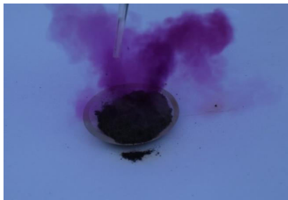
Fig. 2 Rapid reaction initiation using few drops of hot water. The volume of the iodine cloud is directly proportional with the amount of water used.
