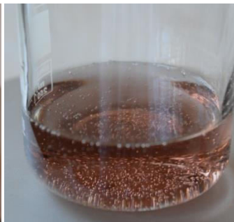
Fig. 3 Once the mixture is heated the oxidation reaction begins, catalyzed by \text{Co}^{2+} , and \text{CO}_2 evolution is noticed.
