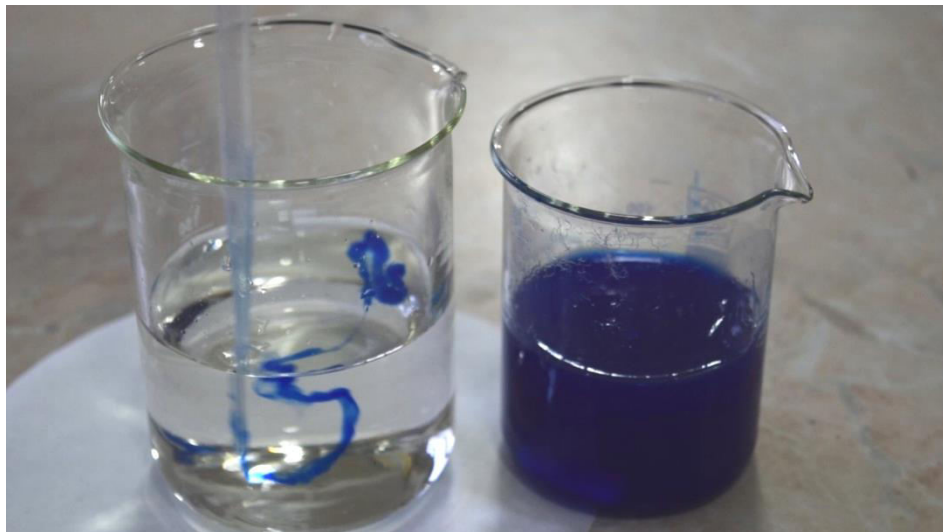
Fig. 3 The cuprammonium solution of cellulose is precipitated using a 10% solution of an acid (in this case \text{H}_2\text{SO}_4 )
