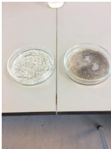
Fig. 2 In this picture you can see the reaction products between hydrochloric and magnesium (right) and hydrochloric acid and zinc (left).
