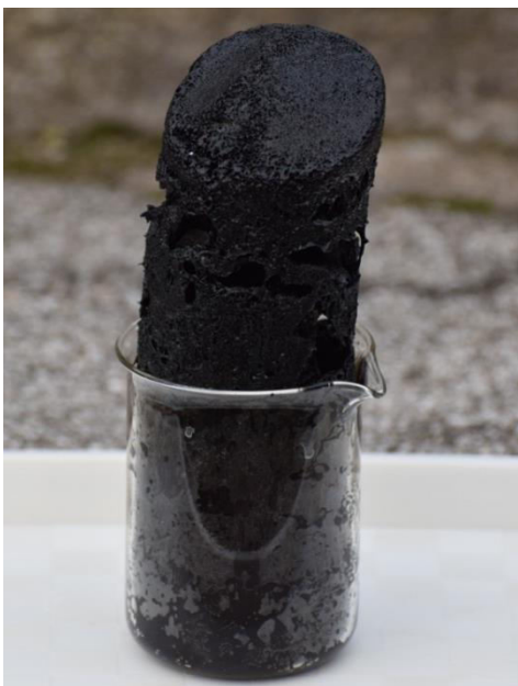
Fig. 2 After a few minutes a black column of carbon emerges from the beaker.
