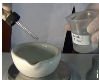
Fig. 2 Diethyl ether is dropped on the honey.
