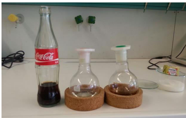
Fig. 3 The sample (left), liquid portion (middle), solid portion (right), the sucrose in the sample caramelized during the distillation, hence the brown colour.
