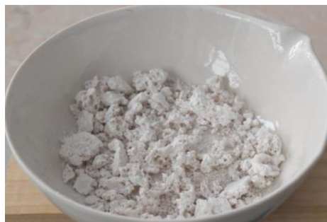
Fig. 2 White solid salt resulted after dehydration of \text{MgSO}_4 \cdot 7\text{H}_2\text{O} .
