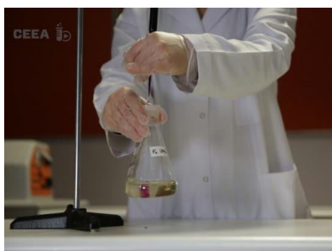
Fig. 3 The shaking continues until the yellow solution turns into a pink color.
