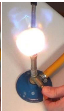
Fig. 3 A yellow flame means a "cold" flame whereas a "blue" one is hot
