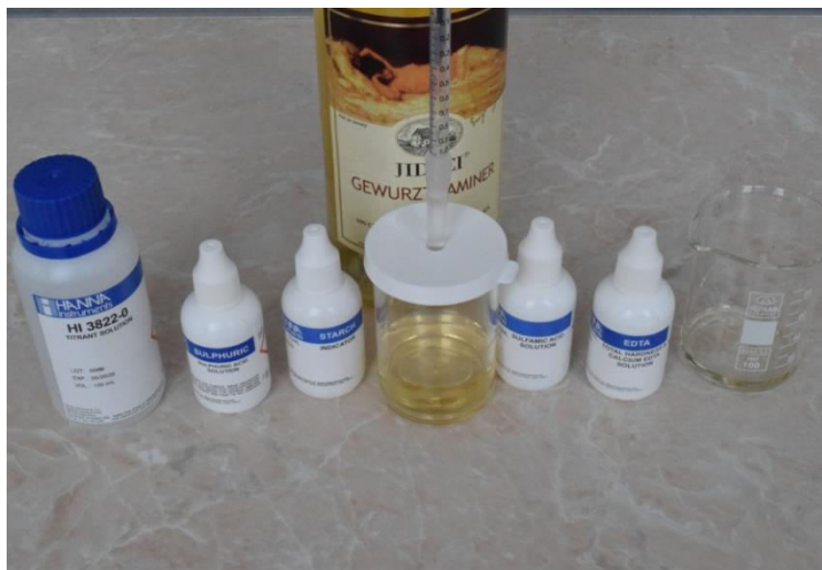
Fig. 1 Wine sample prepared for titration to measure its sulfite content
