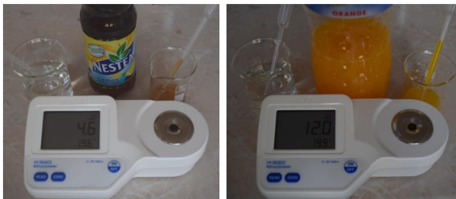
Fig. 1, 2 Some common beverages and their sugar content measured with a refractometer.
