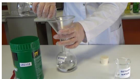
Fig. 2 The water with grease is put into a test balloon with a funnel containing hexane.
