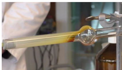
Fig. 2 Combustion tube with sulfur
