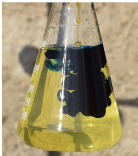
Fig. 5 More concentrated potassium complex (0.25%) with concentrated FeCl_3 (5.0%)
