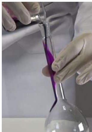
Fig. 2 After being weighted the potassium permanganate is put into a beaker and dissolved with distilled water. This is then added into a 250 mL flask.
