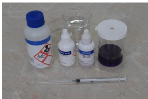
Fig. 2 The end point of the titration process is when the solution turns from yellow to violet. A single drop of titrating solution can cause at the end a dramatic change in color.
