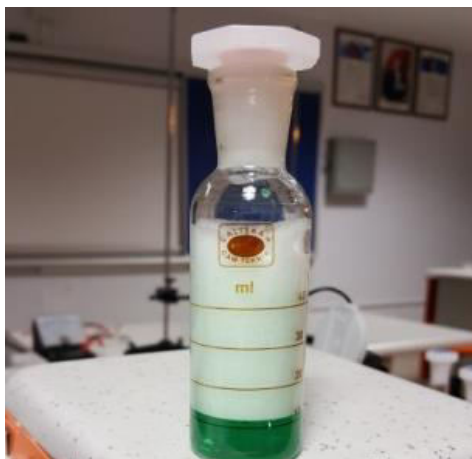
Fig. 7 Checking whether the soap has washing power.
