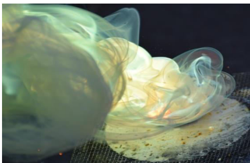
Fig. 2 Initiation of the exothermic reaction between Zn and S with SO 2 evolution
