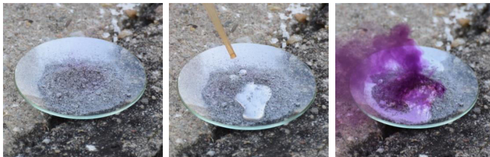
Fig. 1-3 The initiation with hot water of the chemical reaction between 0.5 g powdered Al and 2.0 g \text{I}_2 . After a short period of time the reaction starts and due to the evolved heat, abundant violet iodine vapors are formed.
