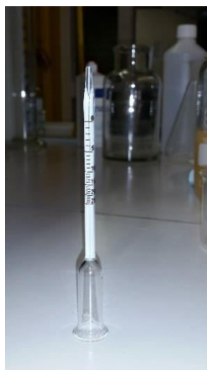
Fig. 3 Measuring the alcohol content with a vinometer
