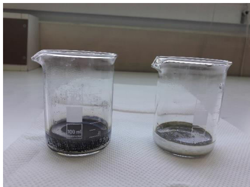
Fig. 1 The silver mirror is formed in the beaker with glucose due to the oxidation of the aldehyde group of C_6H_{12}O_6 which is present in the open -chain form of glucose. The silver mirror is not formed in the beaker with sucrose because sucrose is a disaccharide of glucose and fructose, which does not contain any aldehyde group thus does not oxidize, as it is a non-reducing sugar.
