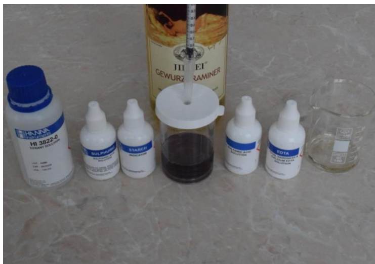
Fig. 2 End point of titration with excess iodine forming a blue complex with starch
