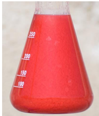
Fig. 3 Ni complex with dimethyl glyoxime, bright red complex obtained when reacting 0.05M \text{NiCl}_2 solution with the chelating agent.
