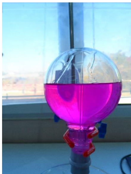
Fig. 2 The mixture turns into fuchsia because of the basicity of ammonia and the indicator phenolphthalein.
