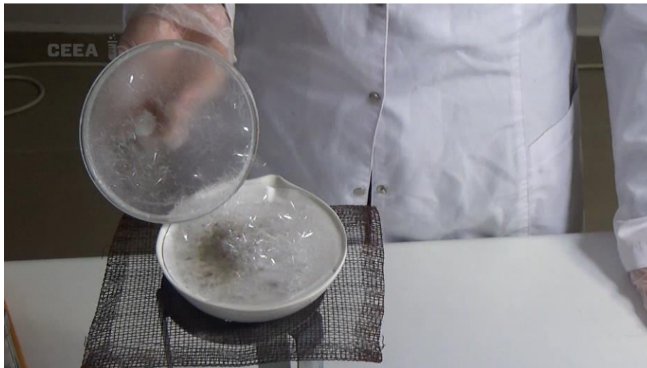
Fig 3. Benzoic acid which is in steam phase hits the surface of the cold funnel and crystallizes.
