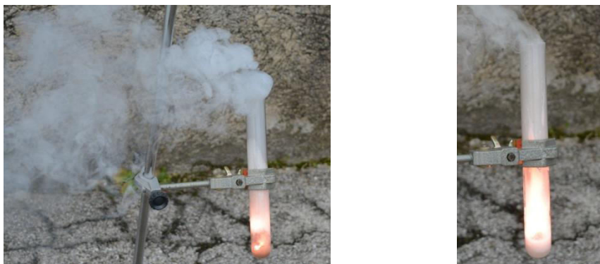
Fig. 1,2 Energetic reaction of molten KClO 3 with sugar (in this case a jelly bear) with a zoomed picture of the reaction site.
