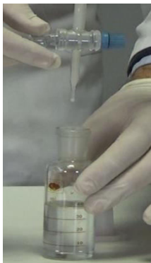
Fig. 1 Slowly dripping soap solution from the hydrometer burette into the sample.
