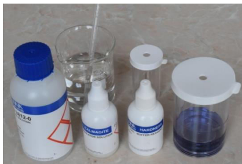
Fig. 2 At the end of the titration the indicator Calmagite is blue and non complexed. All \text{Ca}^{2+} and \text{Mg}^{2+} ions are bind to the EDTA from the titration solution.
