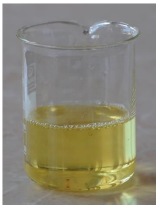
Fig. 5 The solution transferred in a 200 mL beaker after the addition of the 5M NaOH solution (40 mL) is the con-centrated Nessler Reagent.
