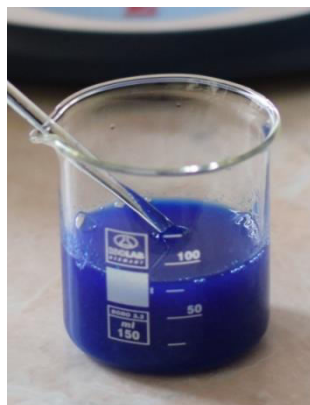
Fig. 3 The precipitate dissolves as concentrated ammonia is added to the copper hydroxide.
