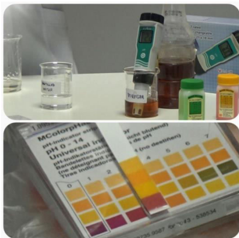
Fig. 2 The measurements taken with pH meter are compared with the indicator measurements and the acidic and basic values of the samples are determined.
