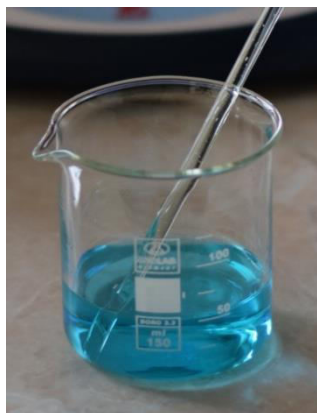
Fig. 1 A 3.84% solution of \text{CuSO}_4 is the starting point for the Schweizer's Reagent synthesis.
