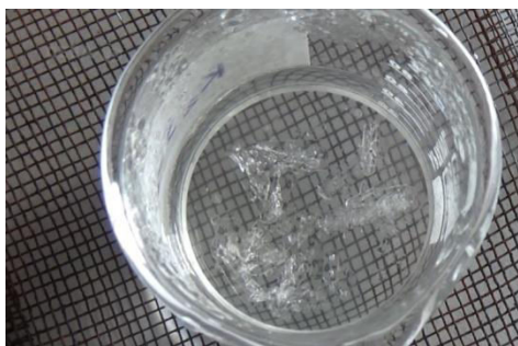
Fig. 3 It is observed that in the solution left to cool down crystals have formed.
