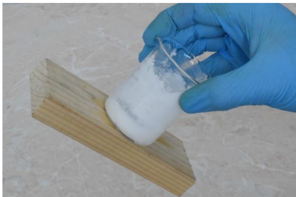
Fig. 1 Barium hydroxide mixed with ammonium chloride is a classical example of endothermic reaction. Spectacular effect is given by the beaker frozen to a moist wooden plate.
