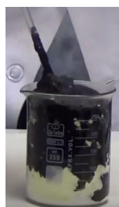
Fig. 4 In just seconds sugar burns, and as a result graphite is observed.
