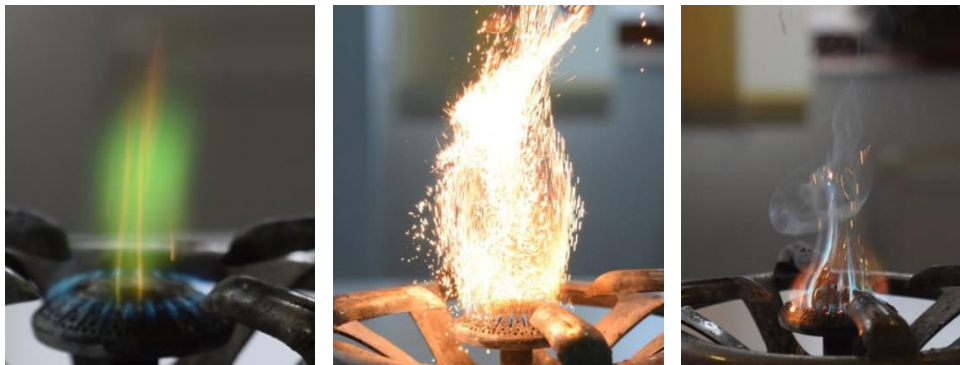
Fig. 1-3 As the sparks are whiter the reactivity of the metal reacting with oxygen is higher. Copper (Cu) left; Iron (Fe) middle; Zinc (Zn) right.
