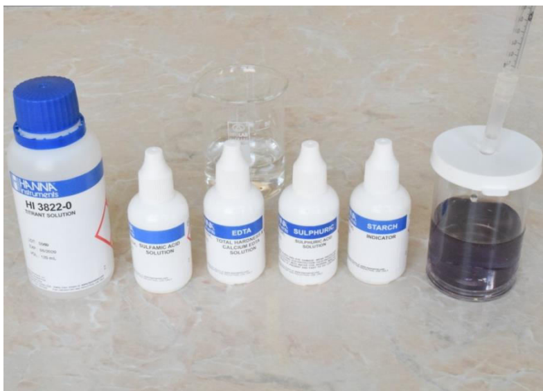
Fig. 2 End point of the titration process for determining sulfites content in water
