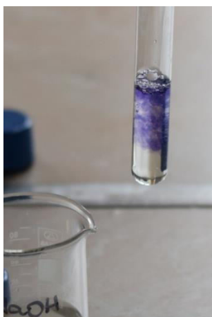
Fig. 3 The biuret test is positive if a violet color appears by adding 1% \text{CuSO}_4 solution.
