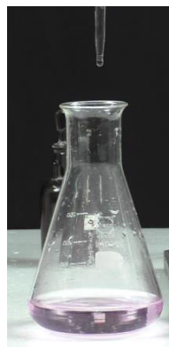
Fig. 3 Reaching the equivalence point.
