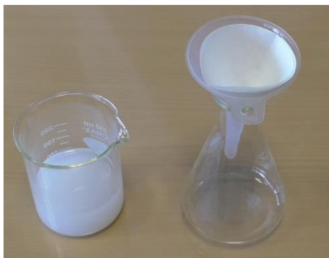
Fig. 1 On the left you see the suspension after the two solutions were added. On the right the Erlenmeyer with a funnel and filtration paper
