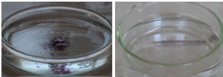
Fig. 2-3 Period 3 metals Mg (left) and Al (right) and their interaction with water
