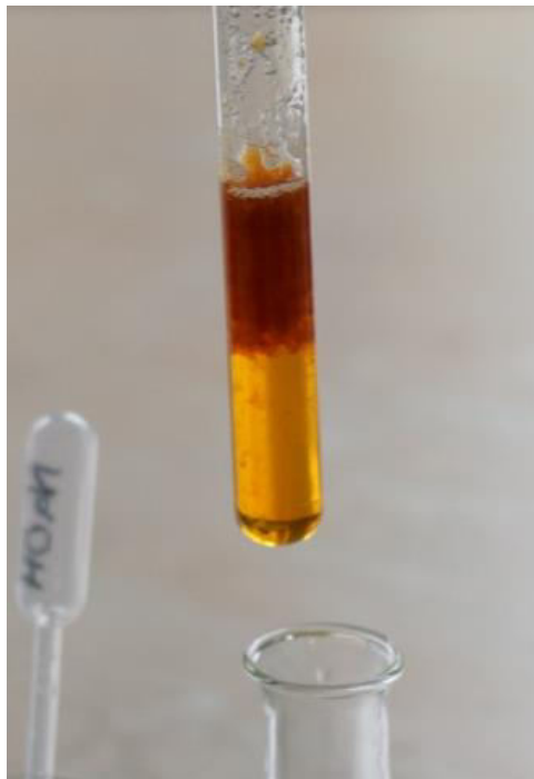
Fig. 4 The addition of the concentrated NaOH (6M) turns the color from yellow to orange.
