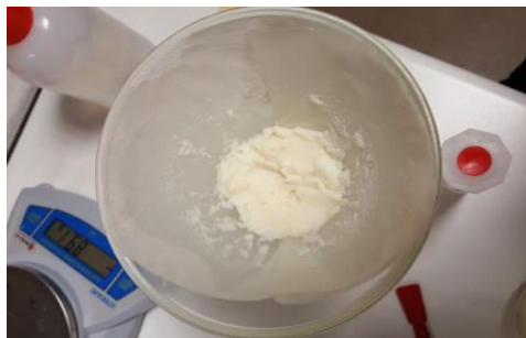
Fig. 4 Wash this paste with thinned NaCl solution and distilled water. Add food coloring and strain it.
