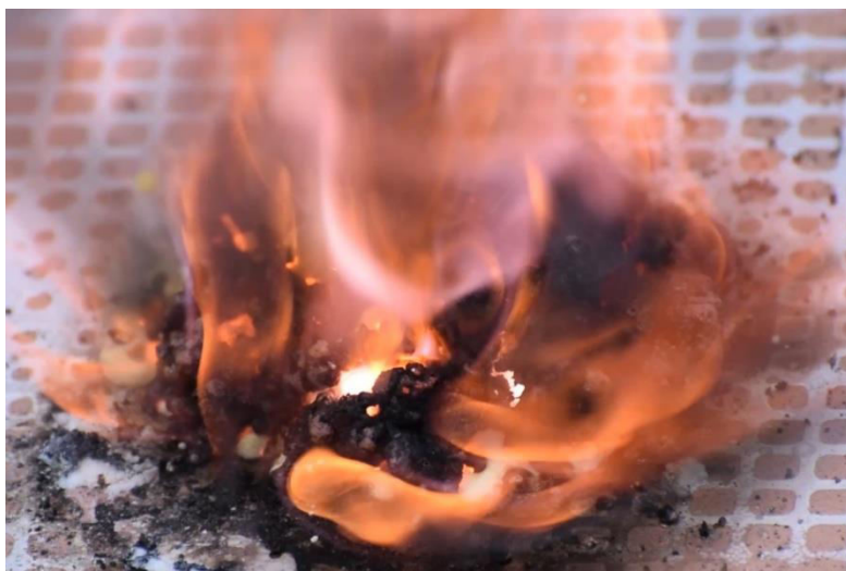
Fig. 1 Exothermic reaction between sugar and potassium nitrate with an abundant evolution of gases.
