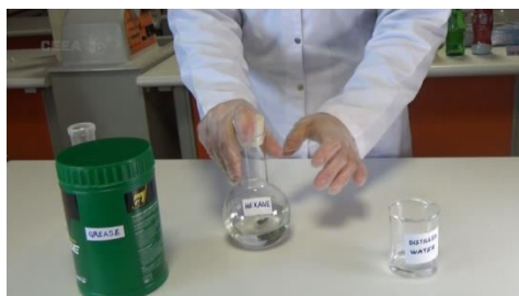
Fig. 3 With the mixture consisting of water, hexane and grease are shook to see its dissolubility.
