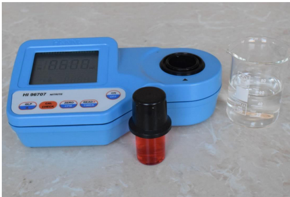
Fig. 1 Experimental setup for nitrites determination. The result shown here is for a solution with more than 0.600 ppm (0.700 mg/l) \text{NO}_2^- . Observe the intense color for a tiny concentration.
