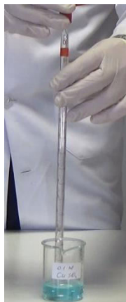
Fig. 1 Put 10mL of 0,1M \text{CuSO}_4 solution with the help of a pipette into a test tube.
