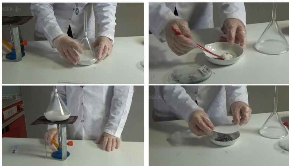
Fig 1. Benzoic acid and carbon dust are mixed in a porcelain capsule, and sealed with filter paper.
