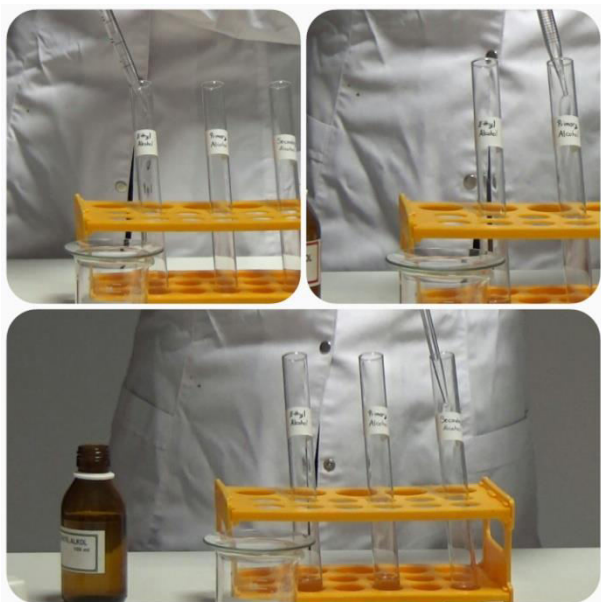
Fig. 1 With the help of a pipette 2ml of Ethyl alcohol, primer butyl alcohol and secondary butyl alcohol are added in test tubes in a row.
