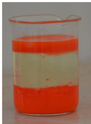
Fig. 4 Further addition of KI dissolves the \text{HgI}_2 precipitate giving the water soluble complex \text{K}_2[\text{HgI}_4]
