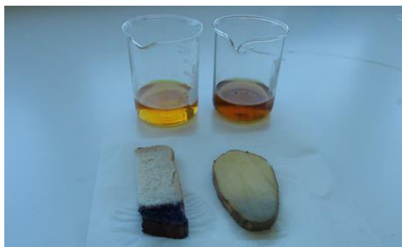
Fig. 1 The color of bread and potato turns into blue after the dip in the iodine solution. This is more obvious in bread because it has a higher content of starch than potato.
