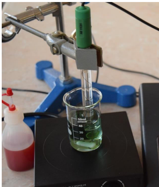
Fig. 2 Experimental setup to record pH change during the titration of \text{H}_3\text{PO}_4 with \text{NaOH}
