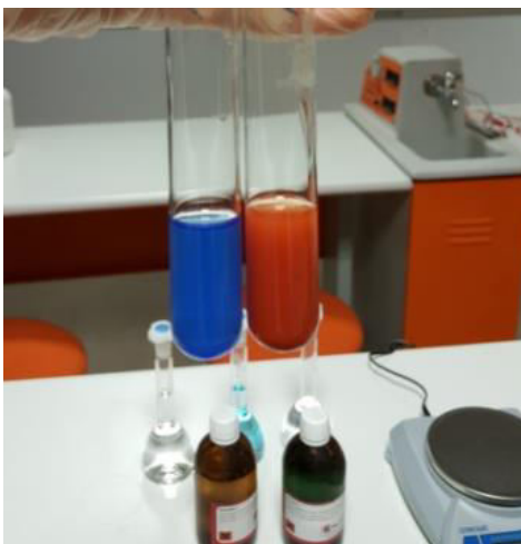
Fig. 2 Keep one as blank probe and add glucose solution in the second one. The brick red precipitate is a positive test for aldoses.
