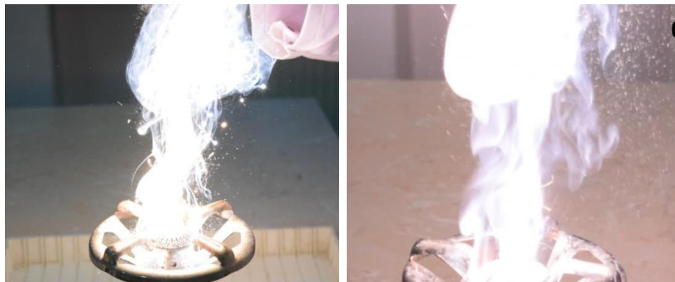
Fig. 4-5 High reactivity (and electrochemical potential) shown by bright sparks formed in the reaction with oxygen shown by Aluminium ( Al - left) and Magnesium ( Mg - right)
