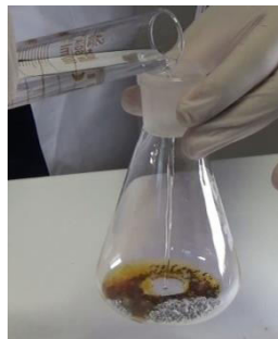
Fig. 3 After the Potassium iodine, and crushed iodine is put in the flask finally, ethyl alcohol is added to the mixture.
