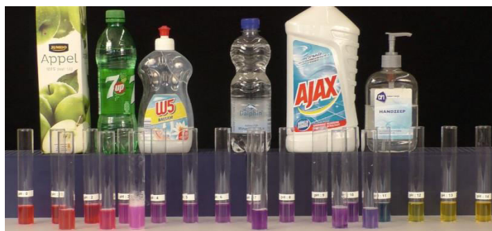
Fig. 3 pH measurement of commonly used products with red cabbage juice.
