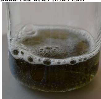
Fig. 4 The most abundant \text{CO}_2 evolution (highest reaction speed) is noticed when \text{Co}^{2+} is oxidized to \text{Co}^{3+} .
