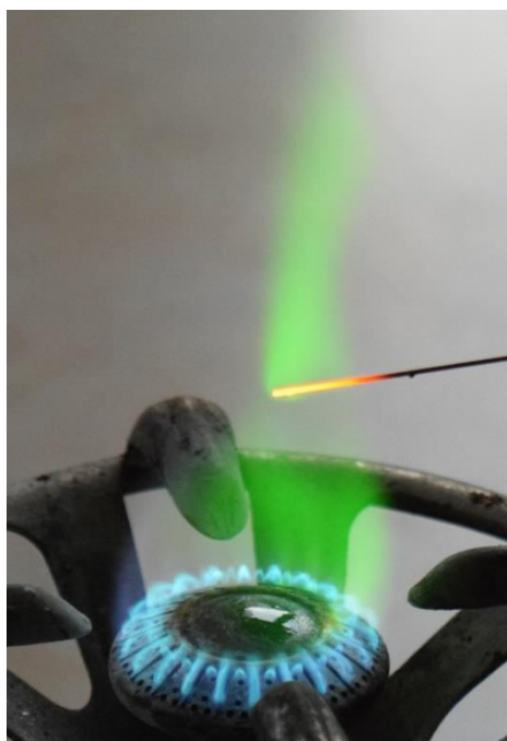
Fig. 3 Green flame of the Tl(I) sample
