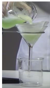
Fig. 7 After the mixture is blended the mixture is filtered with filter paper through a funnel.
