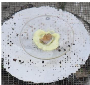
Fig. 1 Place the mixture of Na and S on a disposable watch glass and heat it.
