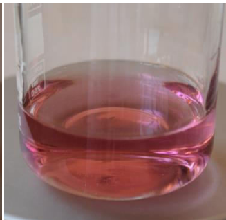
Fig. 2 10 drops of \text{CoCl}_2 5% are added turning the solution pink. If the solution is cold no reaction is observed.
