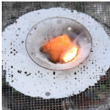
Fig. 5 Hot sodium sulfide generated in the reaction. Sometimes the used watch glass or the crucible breaks into pieces due to the generated hot.
