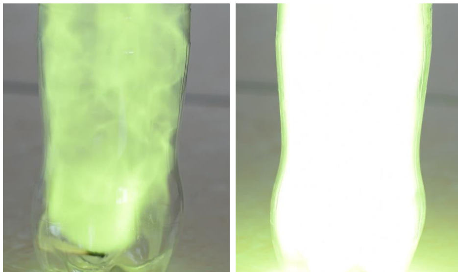
Fig. 4 Two mL of the reaction product, spread in the interior of a 1.5 or 2L PET bottle, burns rapidly (sometimes with an explosion) once ignited.
