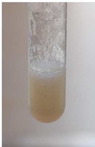
Fig. 3 Albumin denatured by heat
