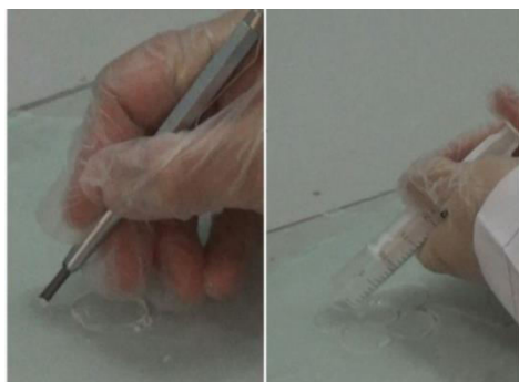
Fig. 3 After covering the surface of the glass with paraffin, a figure is drawn with a metal pencil. Then HF acid is applied on the figure covered with paraffin.
