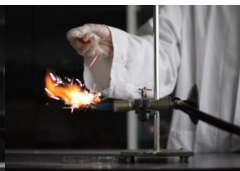
Fig. 3 Setup for the experiment with magnesium powder
