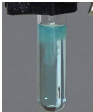
Fig. 2 1mL (20 drops) of \text{NH}_3 solution is dropped in the test tube with a dropper into the \text{CuSO}_4 solution carefully. Continue to drop \text{NH}_3 bit by bit, into the \text{CuSO}_4 solution in the test tube.
