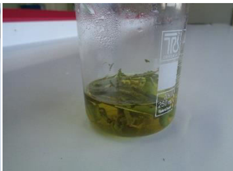
Fig. 2 The pigments and the aroma compounds are transferred from the tea leaves in the solvent.
