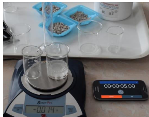
Fig. 3 Mass loss after 5 seconds from the reaction starts when \text{CaCO}_3 was 5 mm marble chips. 0.015g \text{CO}_2 evolved
