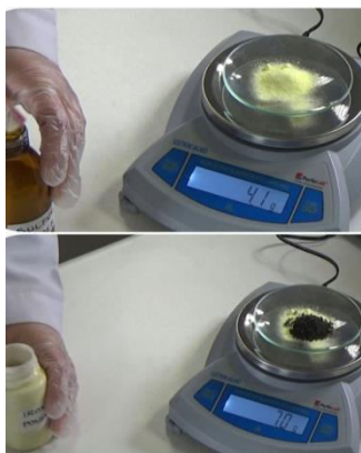
Fig. 1 After the watch glass is tarred, sulphur and iron powder are weighed in a row and mixed.
