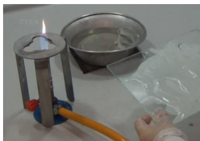
Fig. 2 The section of glass that the hydrofluoric acid is in contact with reacts with the silicium dioxide in glass and erodes the web like structure of it.
