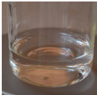
Fig. 1 A 10% Seignette salt solution is treated with an equal volume of 15% \text{H}_2\text{O}_2 . No reaction is observed even when hot.
