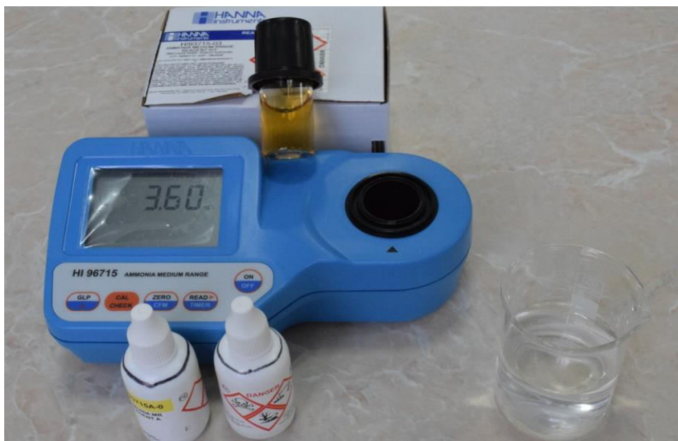
Fig. 1 Very sensitive measurement -positive reaction when a tiny crystal of \text{NH}_4\text{Cl} is dropped in a glass of 250 mL of water which is then analyzed.
