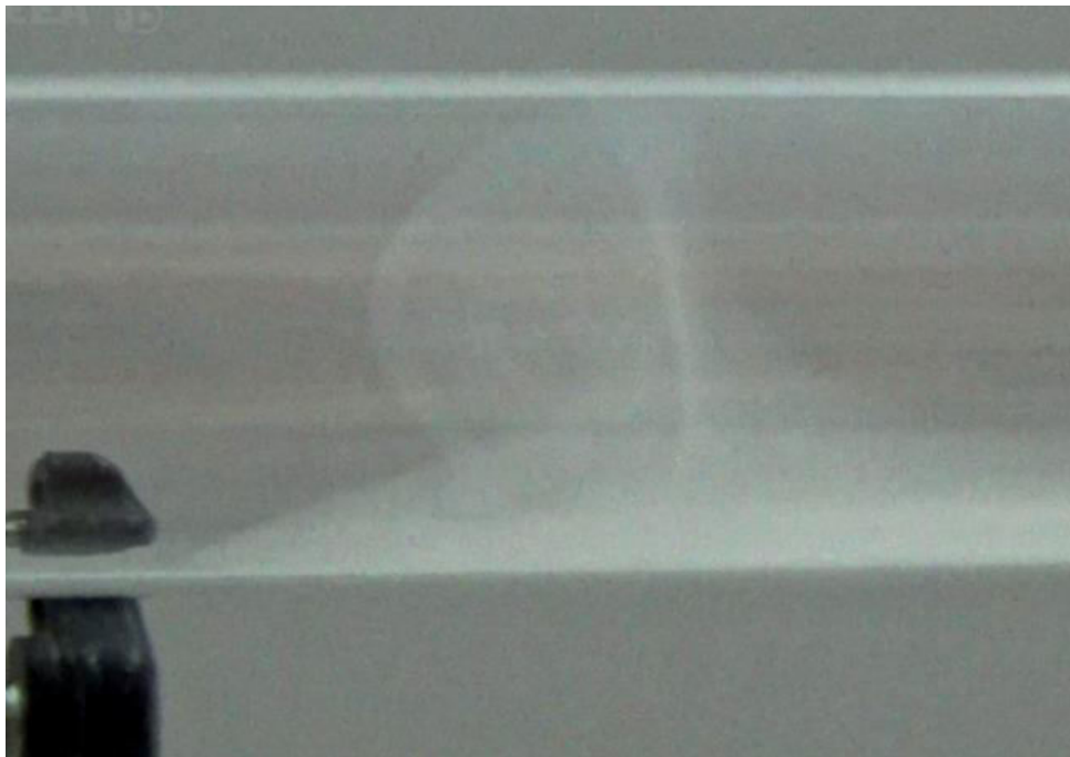
Fig. 3 Due to the gas that has spread through the tube a white cloud is observed. This cloud is ammonium chloride [ \text{NH}_4\text{Cl} ].
