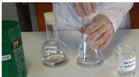
Fig. 1 The grease is taken with a spatula and its degree of dissolubility is observed.
