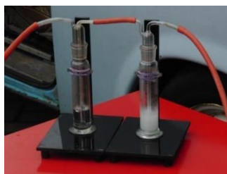
Fig. 3 SO 2 and CO 2 detection.
