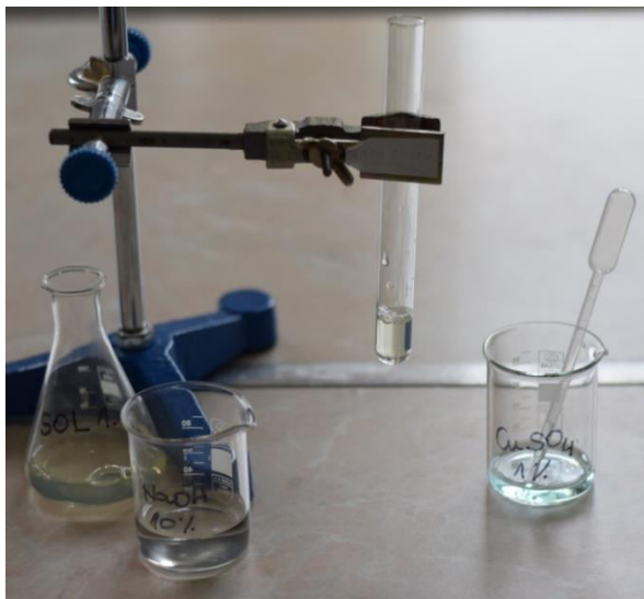
Fig. 1 To perform the biuret test take 3-5 mL of protein solution in a test tube, prepare a 10% NaOH solution and a 1% \text{CuSO}_4 solution.
