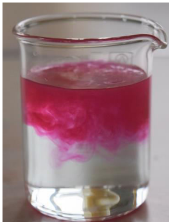
Fig. 1 A 1% dimethyl glyoxime solution dropped over a 0.015M \text{NiSO}_4 solution. The chelate is formed in the upper part due to a lower density of the oxime solution.
