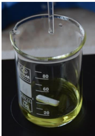
Fig. 1 \text{Cl}^- containing solution treated with \text{K}_2\text{CrO}_4 ready for titration with silver nitrate.
