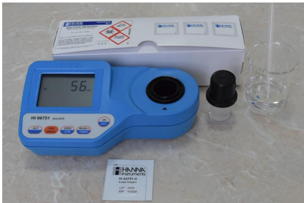
Fig. 1 Experimental setup for sulfates analysis. Observe the turbidity of the analyzed water sample (at a measured level of 56 mg/L)
