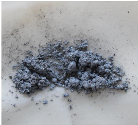
Fig. 2 Silver acetylide freshly filtrated.
