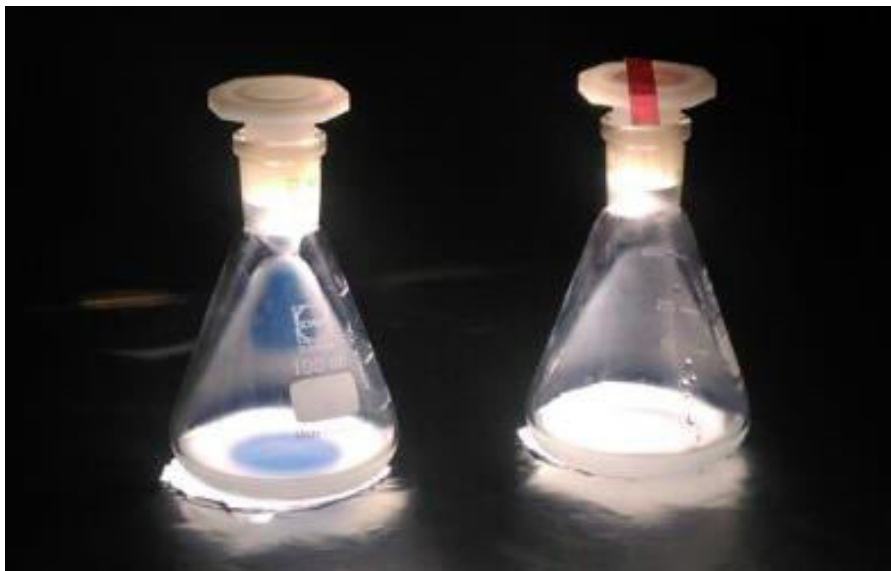
Fig. 1 Photo induced bromination of n-hexane
