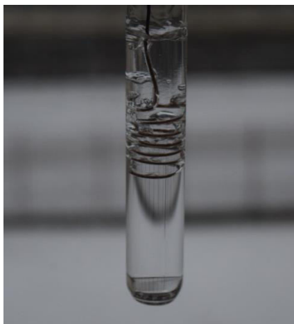
Fig. 6 Hot oxidized copper wire immersed in ethanol
