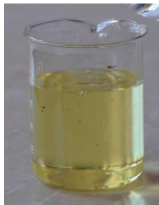
Fig. 6 The Nessler Reagent ready to be used in the identification process of the ammonium ions (after diluted to 200mL with distilled water).
