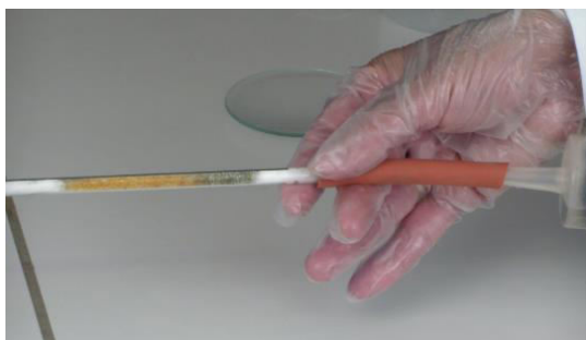
Fig. 3 The colour turns from orange to green upon contact with alcohol vapour.
