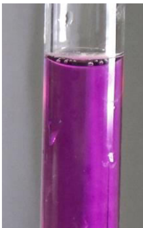
Fig. 3 Finally, it is completed by adding distilled water until the line, in which produces 0.01 molar potassium permanganate solution.
