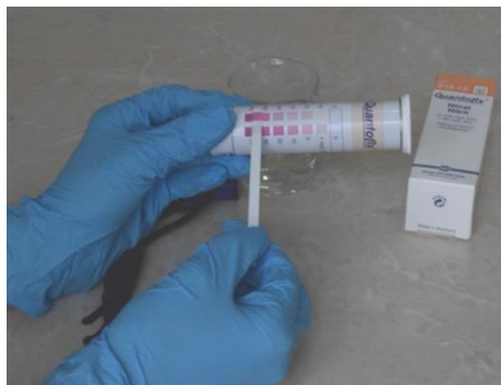
Fig. 2 Comparing the reactive zone with the scale provided allows semiquantitative measurements
