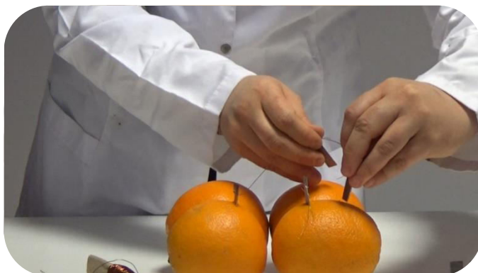
Fig. 2 The plates must be put in the oranges in Cu-Zn-Cu-Zn order and must be connected with copper wire to each other.
