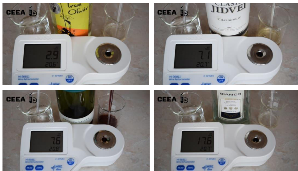
Fig. 1-4 Sugar content measurement of four different types of wines from different countries.
