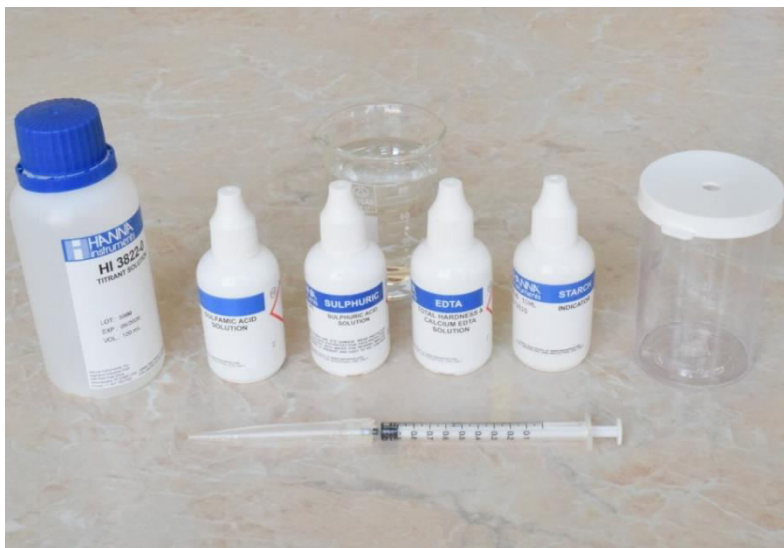
Fig. 1 Titration experimental setup for the measurement of sulfites in water
