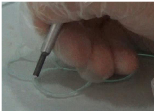
Fig. 5 As a result of the glass and HF reaction, the composed sandy like waste is cleaned with a metal pen.
