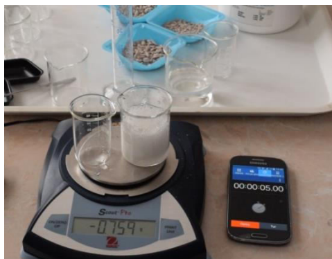
Fig. 2 Mass loss after 5 seconds from the reaction starts when \text{CaCO}_3 was powdered. 0.759g \text{CO}_2 evolved
