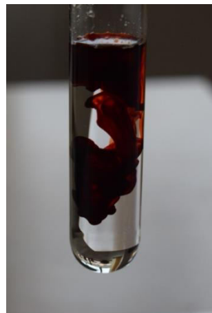
Fig. 3 If \text{FeCl}_3 is 3% when added a 1% solution of KSCN it becomes very dark.
