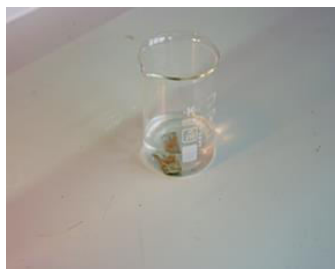
Fig 2. The copper strip quickly becomes coated with a bunch of elemental silver.
