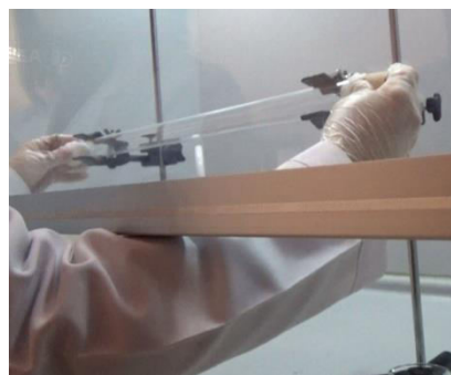
Fig. 2 The cotton which HCl and \text{NH}_3 were dropped are screwed on either end of a glass tube and the spreading of the gas is observed.
