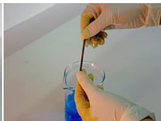
Fig. 3 We observe the color change of the iron nail due to the deposition of Cu onto the iron nail.
