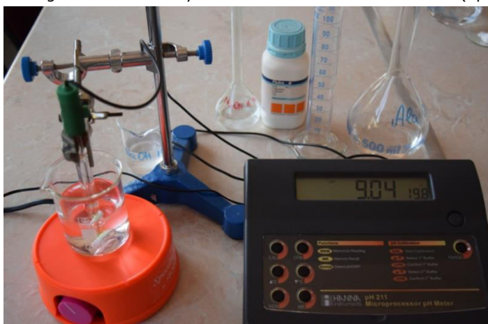
Fig. 2 Experimental setup for measuring the buffer properties of amino acid solutions (0.1M) when strong alkali base is added. Ala 0.1M treated with 1 mL of NaOH 1M ( \Delta\text{pH}=1.79 ).
