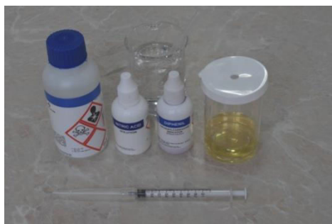
Fig. 1 Experimental setup for chlorine determination after adjusting the pH with nitric acid solution.
