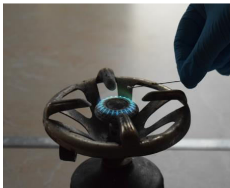
Fig. 2 Tl(I) sample analysis in flame using a previously cleaned pencil lead.
