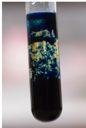
Fig. 3 Dropping K_4[Fe(CN)_6] 3% over a 0.25% FeCl_3 solution gives a precipitate.
