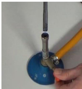
Fig. 1 Lighting up the gas burner
