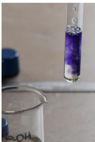
Fig. 4 Further addition of \text{CuSO}_4 gives a more intense violet color.
