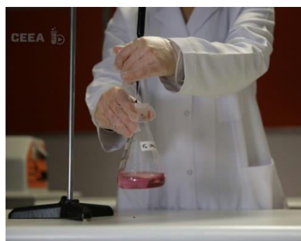
Fig. 2 A pink color is seen, when the equivalent point in titration is exceeded.
