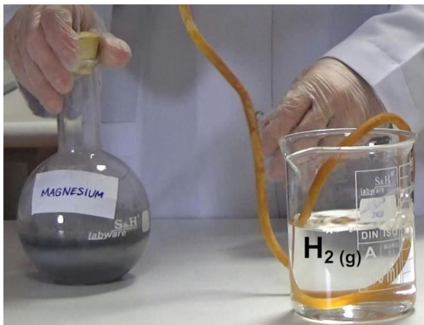
Fig. 5 As a result of the reaction of carboxylic acid with active metals, when formic acid is added, it is observed that \text{H}_2 gas will be released.
