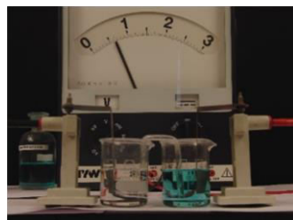
Fig. 3 Daniell cell in action.
